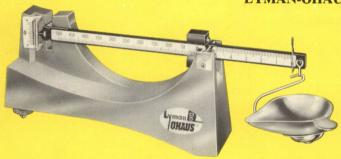
Designed specifically for the reloader . . . . this new Scale has a guaranteed sensitivity of one tenth of a grain. Its high capacity of up to 505 grains, permits the heaviest charges and even bullets to be weighed. Exclusive Lyman magnetic damping assures unsurpassed ease and speed, while genuine agate bearings provide dependable lifetime service.
