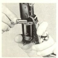
1. Pour a measured amount of powder into each chamber.
