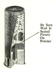
thus improving patterns. Of course, leading is completely avoided with such wads. But their greatest advantage, is extended case life. The abrasive action of the shot on the case mouth is eliminated and we can, in many instances, double the case life over that of a non-sleeved shot charge. Of course, the one-piece wads which combine a shot sleeve are the ultimate in convenience and long case life.
